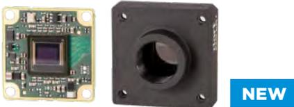
With on-camera ISP: Bare board and S-mount models with BCON for MIPI interface and 5 or 13 MP resolution. Here, specific drivers for NXP's i.MX 8M Mini, 8M Quad, 8QuadMax and NVIDIA's Jetson™ platform are available as a standard.
